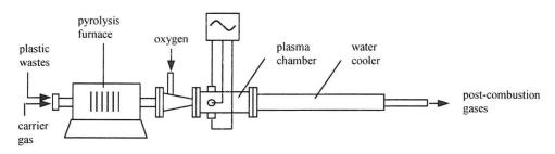
Fig. 1. Schema of the plastic wastes utilization apparatus.
