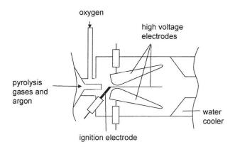
Fig. 2. Schema of electrodes configuration in plasma chamber.
